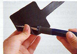
One step insertion and removal of soldering iron tip with the heat-resistant pad
